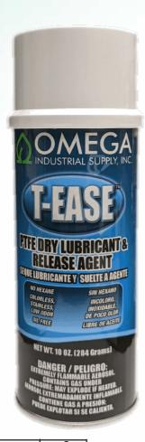
**T-EASE** is a chemically inert, non-oily, non-staining lubricant and release agent that is clean and dry during use. The extremely slick nature of this waxy fluorocarbon will not dissolve away from surfaces and will not melt below 500°F. **T-EASE** repels oil and water, will not attract or hold dust or dirt, and will not become gummy. **T-EASE** is suitable for use as a release agent for rubber, epoxy, phenolic, polyester and other resins.
